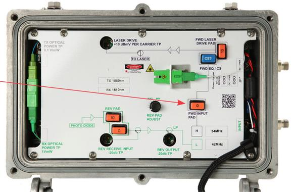
**Note** – For Optimal SNR/MER do not pad here on first stage unless the TIP is > 20 dBmV. For Up Sloped Inputs approximate or calculate Total Composite Power. A few Channels at 22 dBmV at the end of the spectrum with a 12 slope will not require 2 dB Pad.
