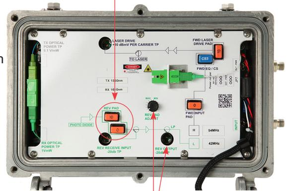
Turn Rev Pad Adjust until Rev Output (-20 dB T.P. = 25 dBmV/Ch)
